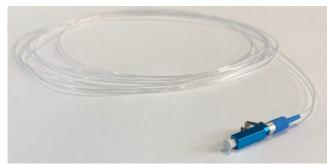
An LC2+ high-temperature connector was chosen due to its ability to withstand the harsh environment inside the autoclave. The feedthrough hermetically seals the ambient environment from the autoclave's inner process environment, using the LC2+ connectors.
