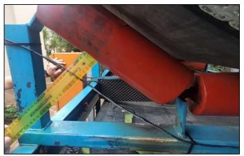
Figure 7. Fibre sensing cable installed for radiated heat test
