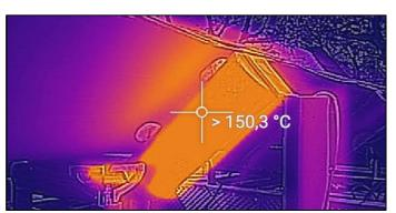
Figure 8. Temperature of idler just after heating sources have been removed
