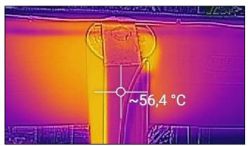
Figure 6. Temperature of idler frame steelwork due to conduction
